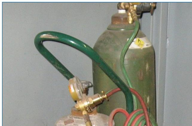
off either the fuel or oxygen first. Check your specific manufacturer's recommendations for the proper valve shutdown sequence. The most important concern is to get both valves closed quickly and to understand any shutdown sequence before an incident occurs.
